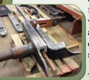
conducted crack testing to check for any further damage before undertaking welding repairs by way of our Lloyds approved fusion welding procedures for cast iron, giving a repair as strong if not stronger than the original material.
