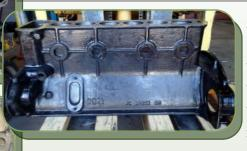
A Belgian customer brought an Alfa SS 6-cylinder block to our Derbyshire workshop for repair. It was in a bad way, with many cracks, holes, and old weld which needed removing and replacing.
