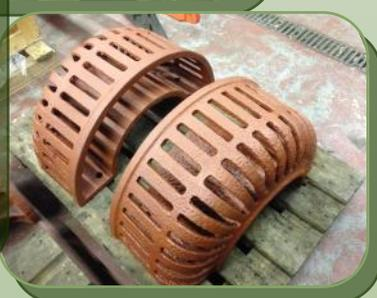
The original baseplate would have been extended and the handle controlling water flow on the same base...as they now had separate bases, it was decided to redesign and make a pattern to what would have been the original shape, and again, the foundry cast up this part, which was welded to the column's base seamlessly!
