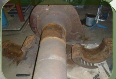
When the water crane arrived in our Derbyshire workshop, all the components were disassembled, shot blasted and crack tested, ready to begin the process of rebuilding.
